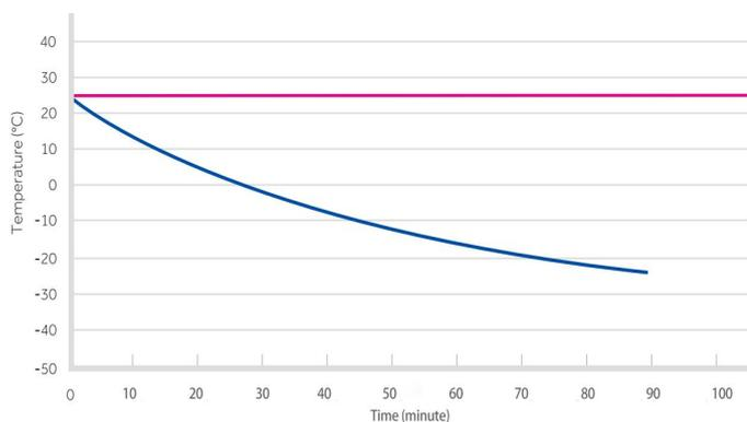
MDF-25V268E Pull Down Test at Ambient
