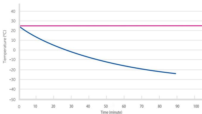
MDF-25V268E Pull Down Test at Ambient
