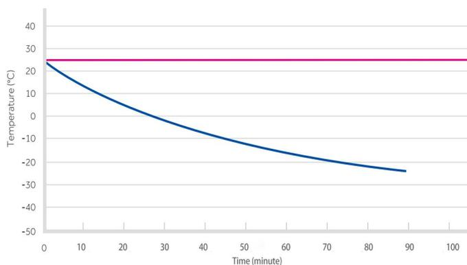
MDF-25V268E Pull Down Test at Ambient
