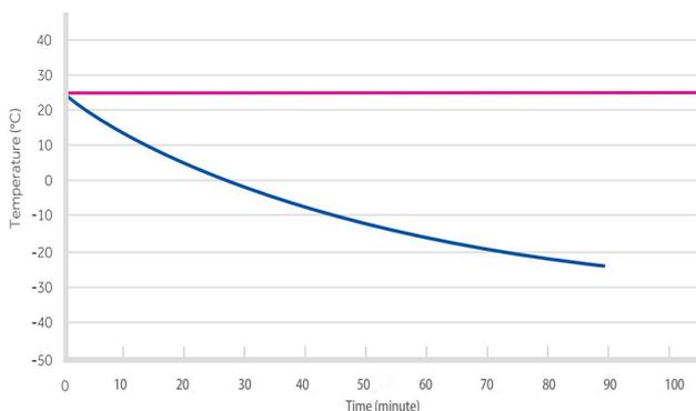
MDF-40V100 Pull Down Test at Ambient
